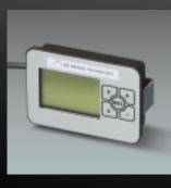
The Sigmagauge LCD is a highly versatile vehicle display, which can be easily configured to meet the OEM's requirements. The backlit, dot-matrix display receives its information over the CANbus, and presents vehicle status and diagnostic information to the operator in clear, easy-to-read icons. The operator, via pushbuttons on the front panel, is also able to select which details are displayed on the screen.
